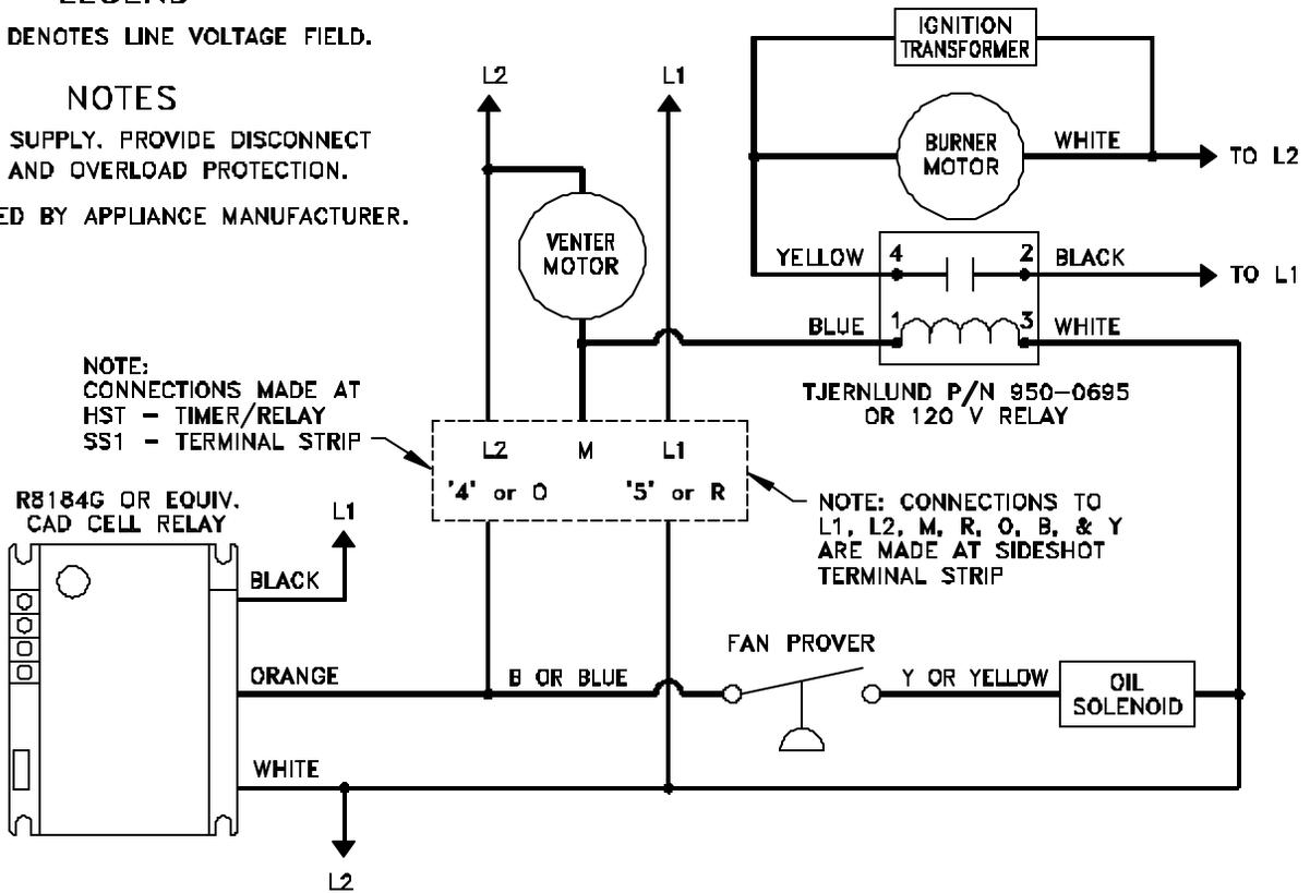
SIDESHOT® OR HST-SERIES WIRED WITH PHELON CONTROL AND BURNER MOTOR POST PURGE KIT
