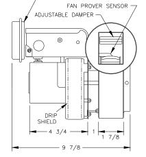
FAN PROVING PRESSURE SWITCH
