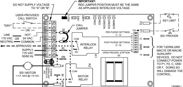
**WARNING:** Disconnect power supply from the SS1C and heating equipment when making wiring connections and servicing the SS1C. Failure to do so may result in personal injury and/or equipment damage. LED #5 (RED) should be off with power removed.
