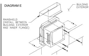
**NOTE:** For mounting on vinyl or lap siding a wood frame with 1" x 1 1/2" on the sides and top and 1" x 2" material on bottom can be utilized on exterior wall. This will provide a flush mounting surface for the hood and a nicely finished look with "J" channel when siding. Inside of frame opening should be 8 3/8" wide by 8" high.
