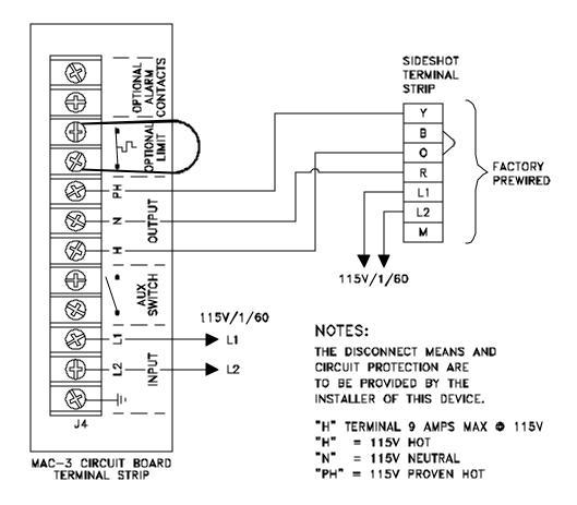
MAC-3 WIRED WITH A POWER VENTER, DRAFT INDUCER OR IN-FORCER WITH A MOTOR GREATER THAN 9 AMPS
