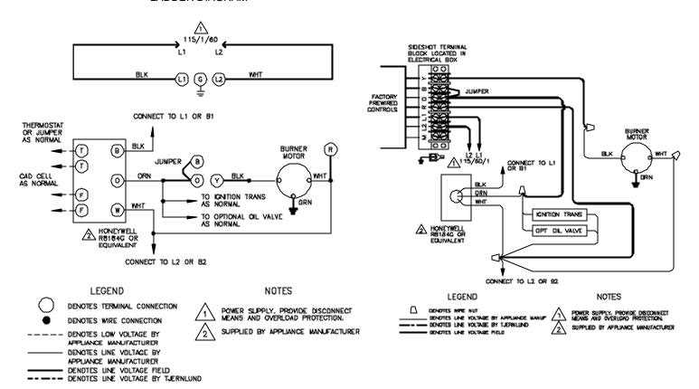
NOTES: The SideShot is always interlocked with the primary control of the appliance. Wire all other furnace/boiler controls as normally done when conventional venting before continuing. Disconnect power from the appliance before attempting to interlock the SideShot.
