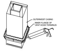
8. Slide the Vent Hood through the wall while taking care installing the rain shield as shown, (See Diagram E). The nuts located on the Vent Hood outermost casing should be facing up when sliding it through the wall. Mount Vent Hood to the exterior using four #8 x 3" wood screws and spacers provided, (See Diagram E). Wall anchors are provided for installation into masonry wall.
